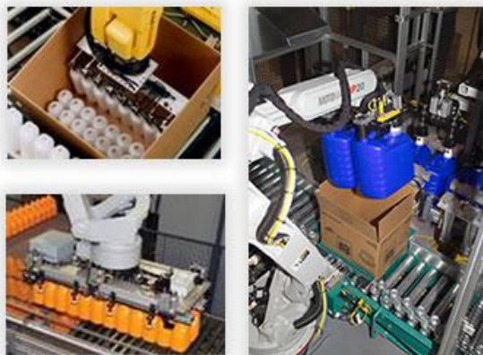
Slika 183: Robotizirano zlaganje plastenk v škatle (Robot Packaging, 2010)
